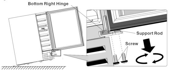
B. Remove the door off the upper hinge and take out the support rod.
